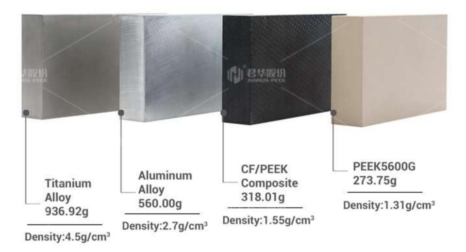
PEEK significantly reduces the overall weight of humanoid robots, enhancing mobility/flexibility while lowering energy consumption and extending operational endurance.
