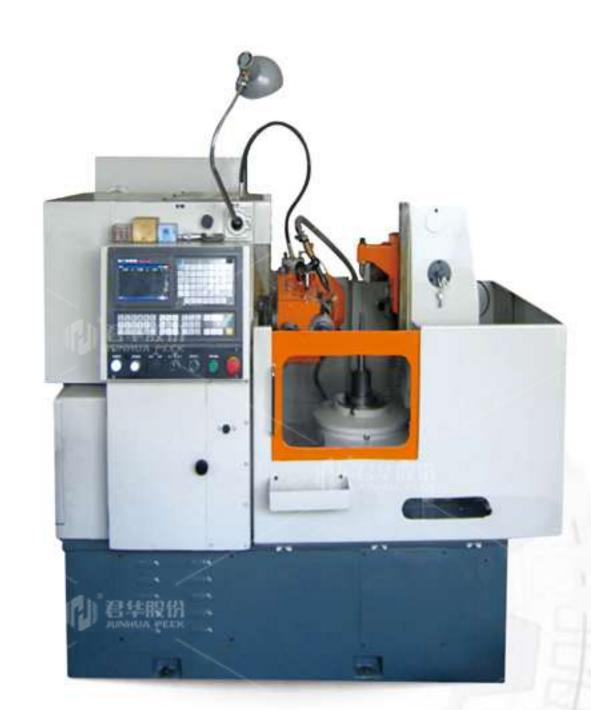
At present, it can process spur gears and helical gears with a module between 0.2-10, a diameter of 520mm and a height of 280mm. It can process PEEK spur gears, PEEK helical gears, PEEK sprockets, PEEK worm gears, PEEK flowers Key gears, etc. and PEEK products with toothed grooves on the circumference, when the processed gears are used to transport liquids, the flow rate can be within plus or minus 0.025L/min.
