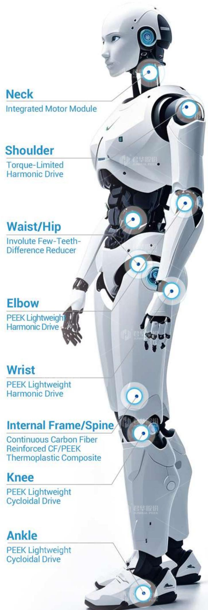
PEEK Harmonic Drive for Humanoid Robot Joints
